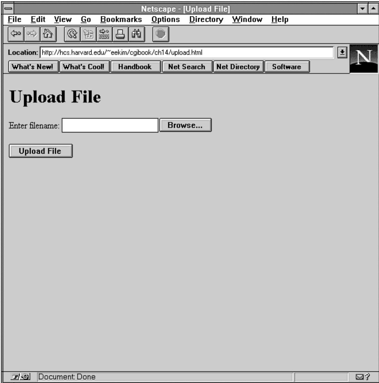
Figure 14.7 : The browser prompts the user to enter the filename of the file to upload.
