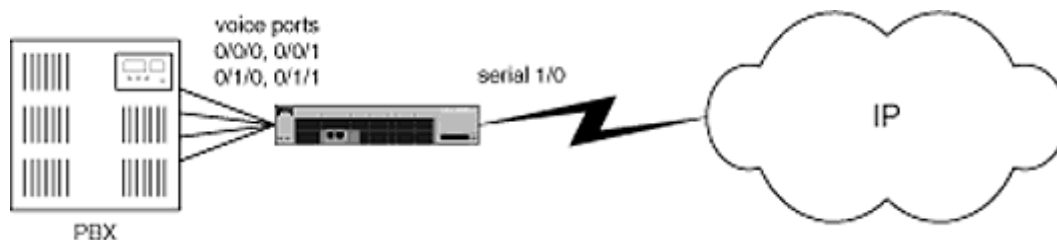
Figure 6-5 PBX connected to a 3640 router with four E&M ports.
