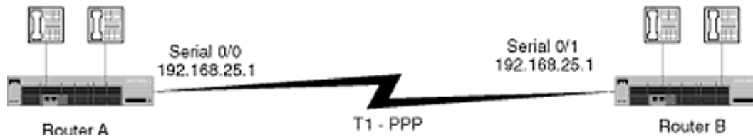
Figure 4-1 PPP compressed RTP.
