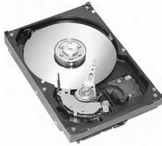
Fig. 3.31 Hard Disk Drive
