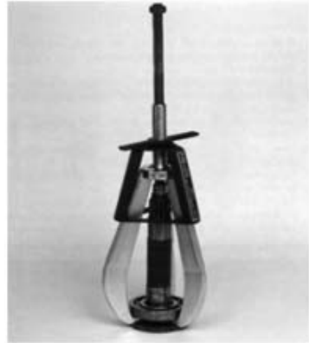
Fig.15.1 - Bearing removal using puller
