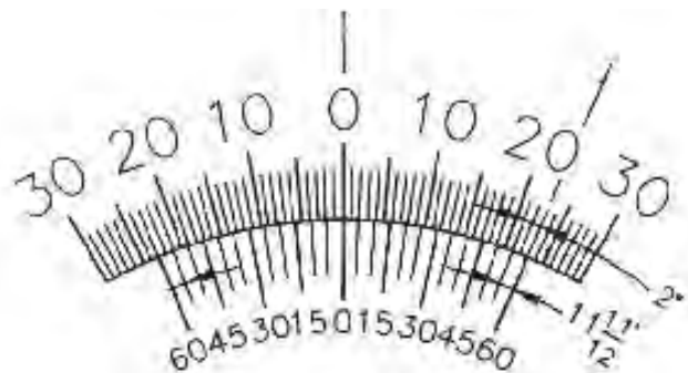
Fig 3.20 Reading with vernier bevel protractor
