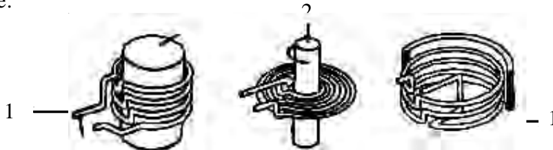
Fig 5.3 Induction hardening 1. Heating coil 2. Metal part
