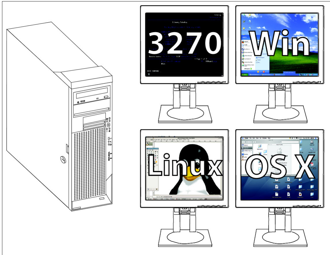
Figure 7-10 On a multi-station system, each client can run a different remote desktop, terminal, or virtual machine
