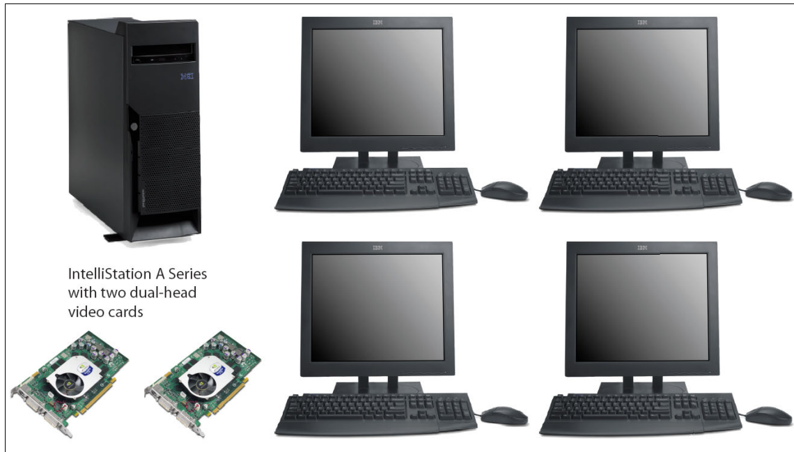
Figure 7-8 IntelliStation A Pro workstation supporting four workstations using two dual-head video cards
