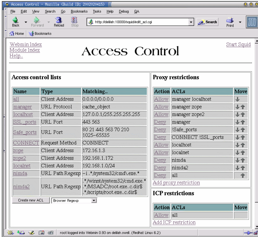
Figure 12.12. Access Control Lists
